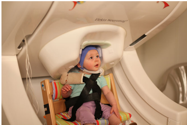
Figure 1 Infant in MEG during measurement. A custom-made adjustable chair was used in order to adjust to the infant's height, placing the infant's head under the MEG sensor array for an optimal position during the recording.
